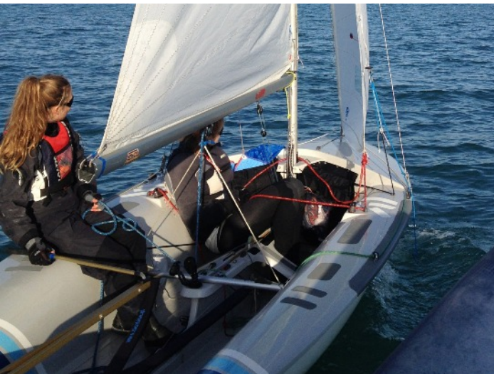
Correct strop length boom is close to the centreline
