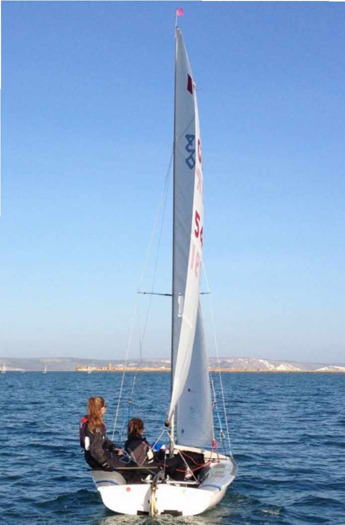
Correct strop length boom is close to the centreline
