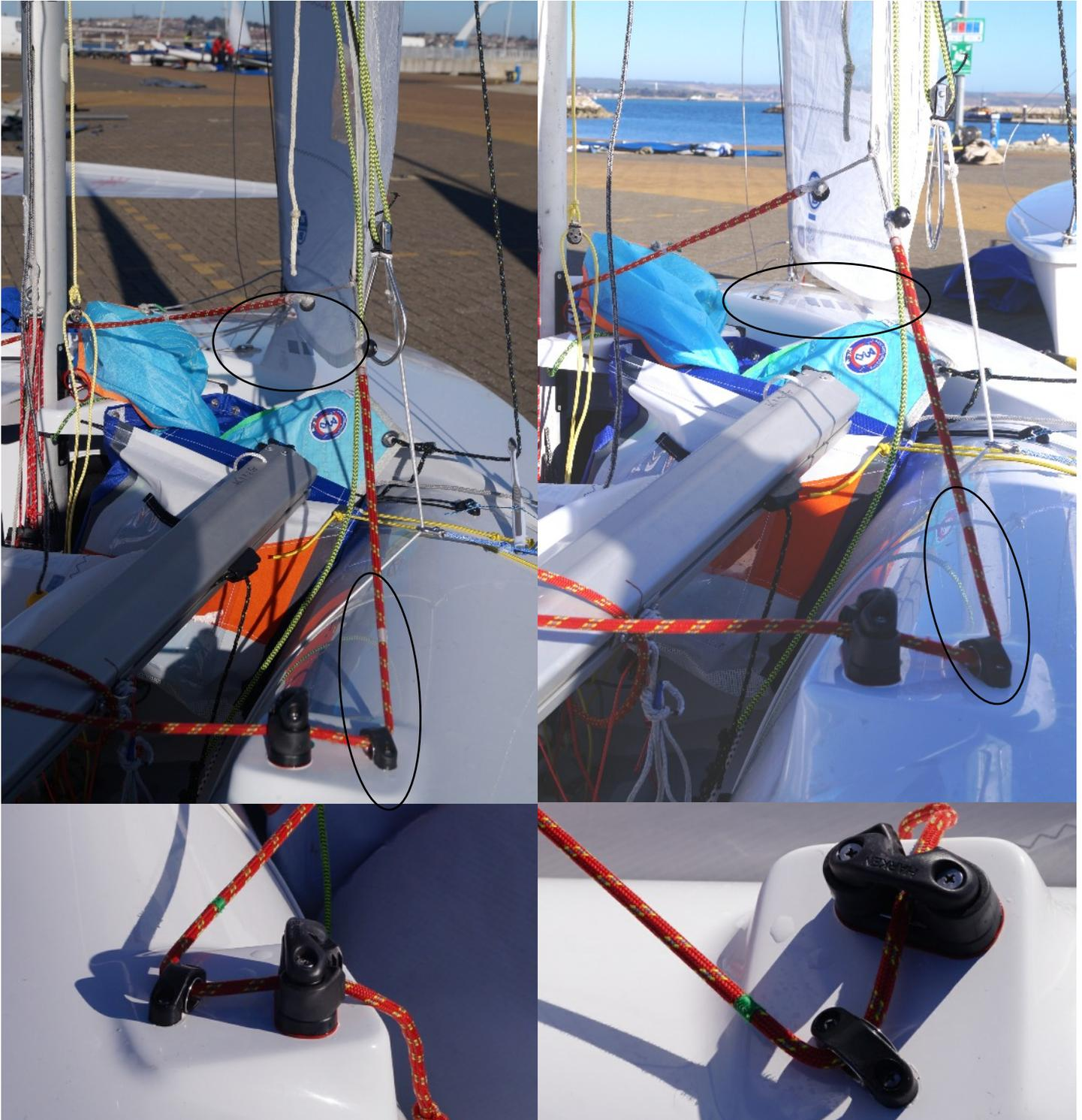
This side shows sheet tension only with no barber hauler. However the barber sheet has been pulled on to take up the slack
